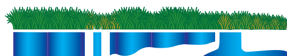
Drip irrigation – uneven and interrupted application due to clogging and rodent damage
