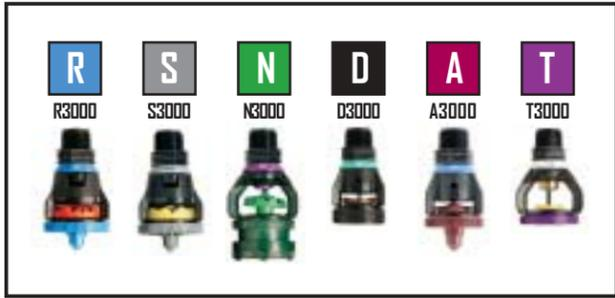
This diagram reflects the modularity of Nelson's 3000 Series Pivot Products. Each sprinkler is made up of an assembly of a cap, plate, body, and nozzle. The 3TN Nozzle is interchangeable with all 3000 Series sprinklers. A variety of connection devices are available to link the sprinkler with a hose or rigid drop.
